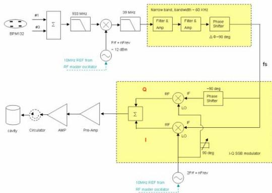
Figure 2: Block diagram of analog mode feedback system. A high power circulator was not installed during this experiment.
