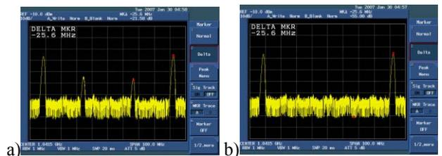
Figure 6: Beam spectrum when 52 bunches are stored in the ring. The digital bunch-by-bunch feedback is turned off (a) and on (b).
