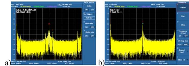
Figure 3: Beam spectrum measured by button electrode when feedback system are turned off (a) and on (b).
