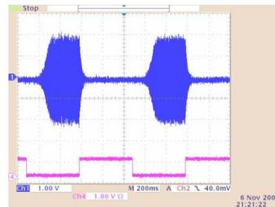
Figure 4: The grow/damp measurement of the instability. The blue line (CH1) shows the longitudinal oscillation and red line (CH4) represents the gate signal.
