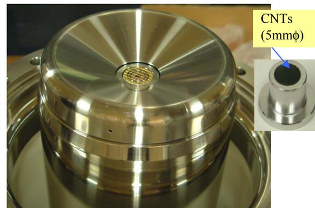
Figure 2: Structure of a field emission electron gun of triode-type with a CNT-cathode. CNTs are contained in a black portion on a cathode shown in a small right picture.
