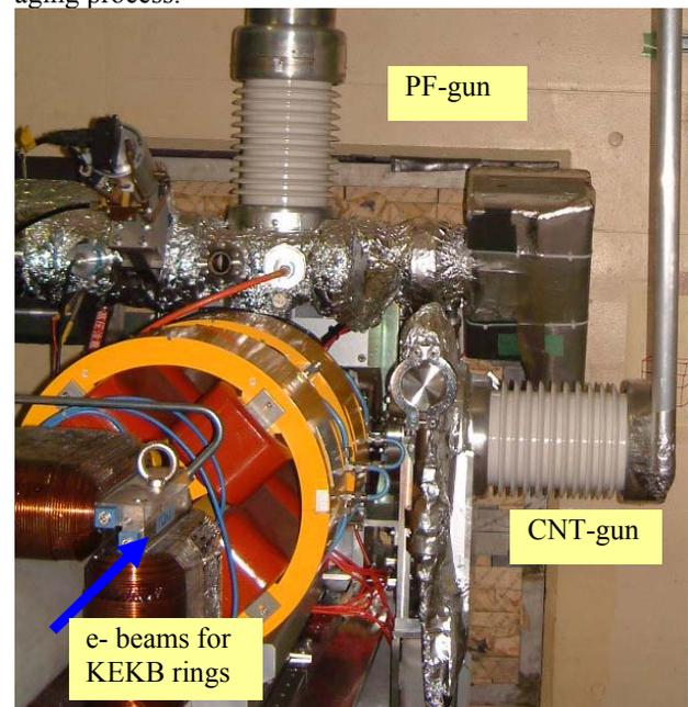
Figure 1: The CNT-cathode gun newly installed in the linac near the existing gun for injection into the PF rings.
