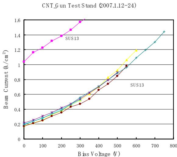
Figure 3: Current densities of the CNT-cathode utilized for the acceleration test.
