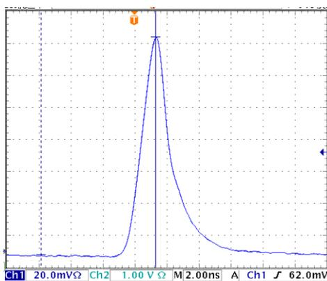
Figure 4: Pulsed beam shape from the CNT-cathode gun.
