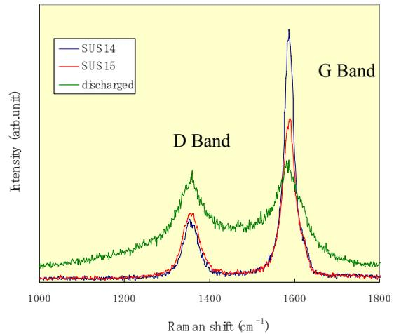
Figure 6: Raman spectra of the CNT-cathode samples.
