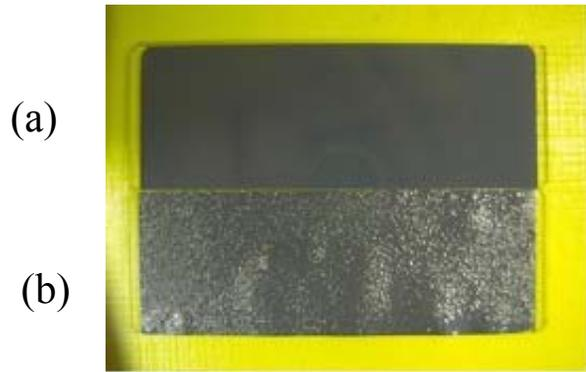
Figure.4 Photographs of carbon layers on slide glasses. Represent an HBC-foil of 370 µg/cm<sup>2</sup> and is for a Cluster-foil of 140 µg/cm<sup>2</sup> made by the CADAD method.
