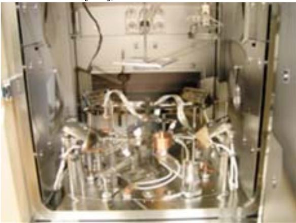
Figure.3 Arc-discharge evaporation-source in EBX-2000C cryo-vacuum pump apparatus.
