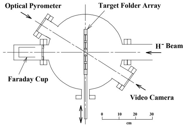
Figure 1: Target chamber
