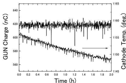
Figure 7: Time trend of the beam charge and the cathode surface temperature with the beam charge feedback system.
