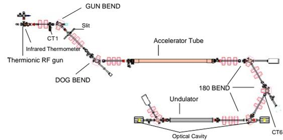
Fig.1 Schematic view of the KU-FEL system
