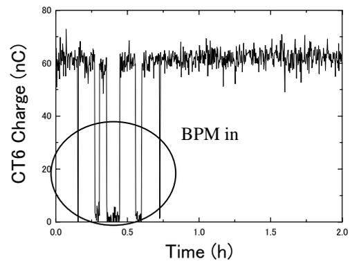
Figure 8: Time trend of the beam charge at 180-bend section with the beam charge feedback system. The zero charge events, "BPM in", correspond to the beam position monitor interrupts the beam at the upstream of the beamline.
