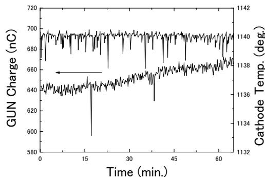
Figure 5: Time trend of the beam charge and the cathode surface temperature with the temperature feedback system.
