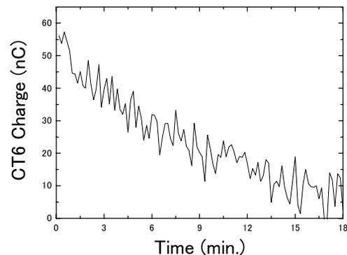
Figure 4: Time trend of the beam charge at 180-bend section without a feedback system.
