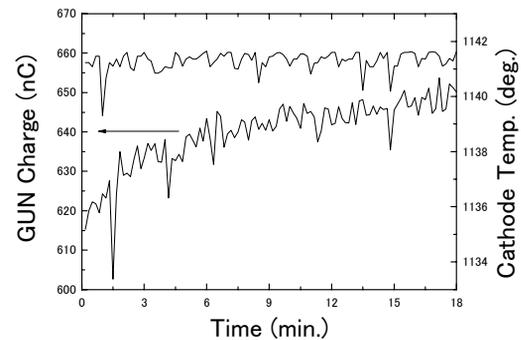
Figure 3: Time trend of the beam charge and the cathode surface temperature without a feedback system.
