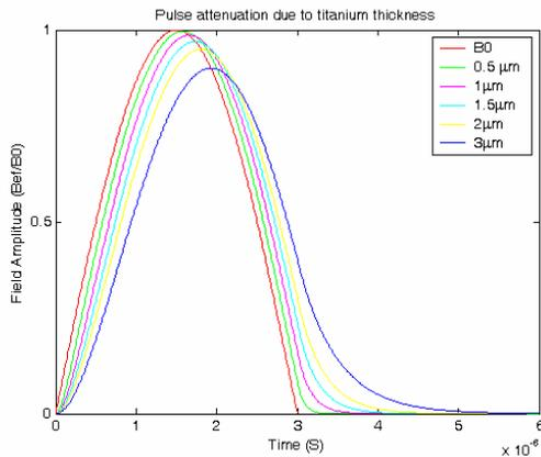
Figure 3: Injection kicker pulse attenuation for various coating thickness
