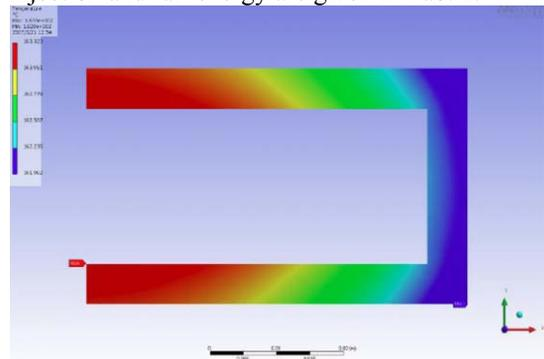
Figure 5: Temperature distribution for  $1 \mu\text{m}$  titanium layer thickness.
