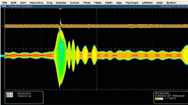
Figure 3: Beam Position signal and feedback signal from kicker cavity of Timing adjustment
