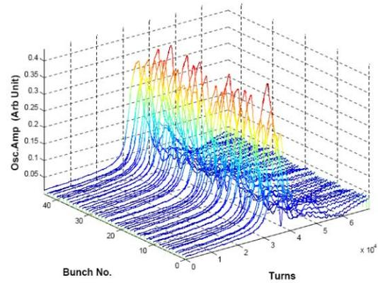
Figure 6: Oscillation record in time domain
