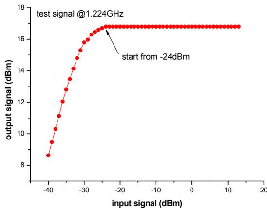
Figure 4: Amplitude response of limiting amplifier
