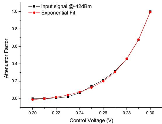
Figure 2: Relationship of Control voltage and Attenuator Factor
