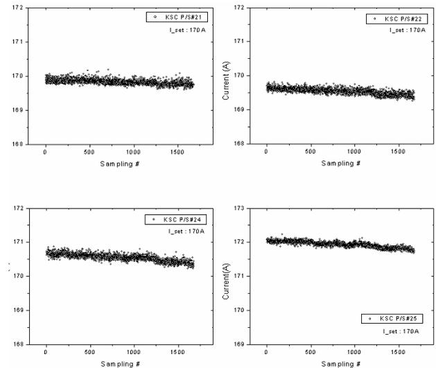
Figure 4: One part of monitoring results for magnet power supplies has been found to be quite stable and capable of saving process variables
