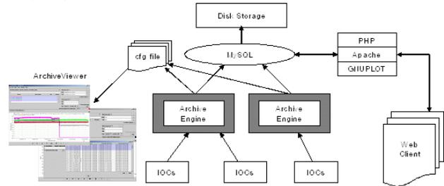
Figure 2: Schematic Architecture of PEFP data acquisition. The left side of an archive engine shows the data storage of a file form and the right side shows the web interface through database.
