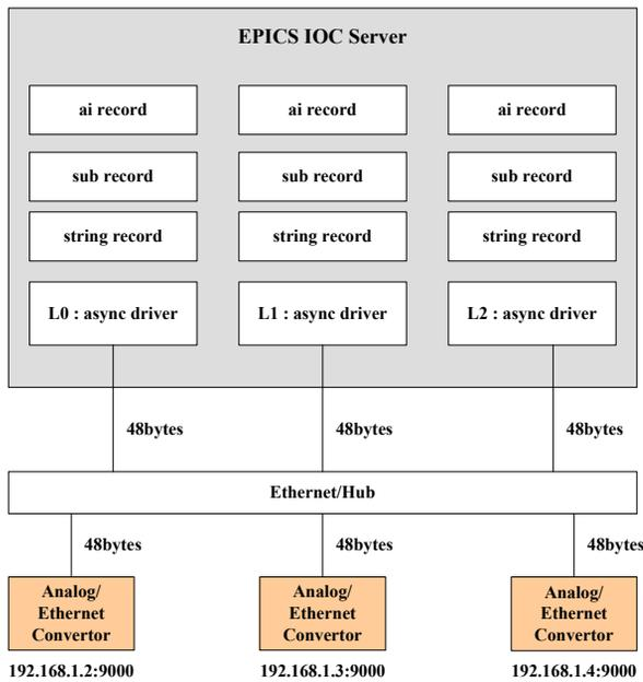
Figure 1: Overall block diagram to monitor DTL Magnet Power Supply System
