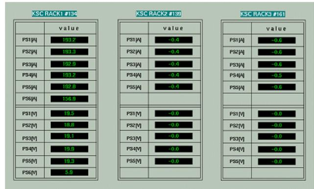
Figure 3: EDM screen that monitors the entire magnet power supplies of analog interface.
