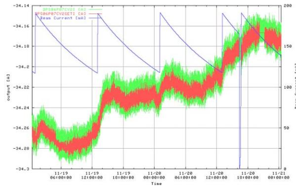
Figure 7: The current change of one specific vertical corrector (7CV2) used in the orbit feedback for two days with the compensation of BPM chamber motion.
