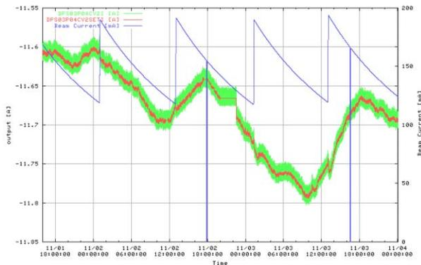
Figure 3: The current change of one specific vertical corrector (4CV2) used in the orbit feedback for two days with the compensation of BPM electronics gain.
