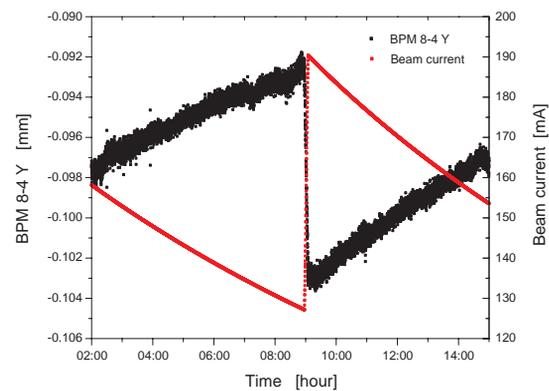
Figure 1: The vertical reading change of a BPM when the beam is re-filled. The red line represents the beam current.
