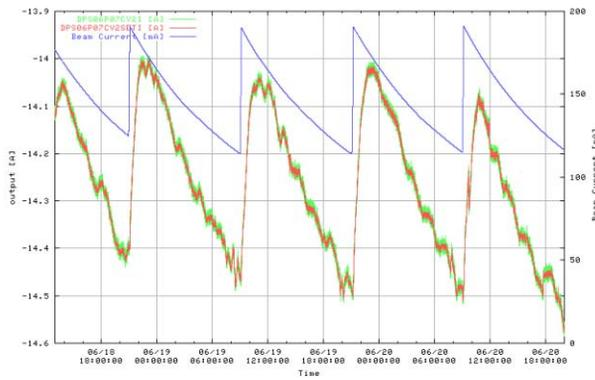
Figure 6: The current change of one specific vertical corrector (7CV2) used in the orbit feedback for two days without the compensation of BPM chamber motion. The definitions of colored lines are the same as in Figure.
