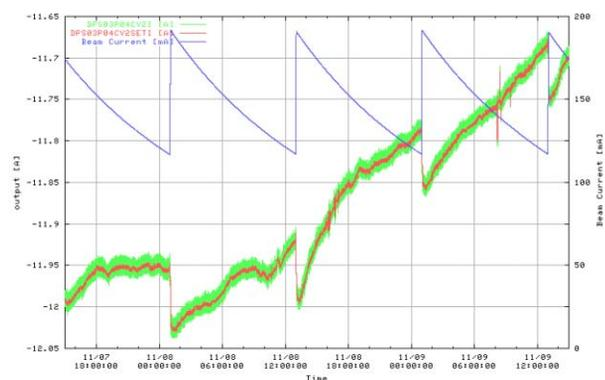
Figure 2: The current change of one specific vertical corrector (4CV2) used in the orbit feedback for two days without the compensation of BPM electronics gain. The blue line, the red line, and the green line represents the beam current, the set value of MPS, and the reading value of MPS, respectively.
