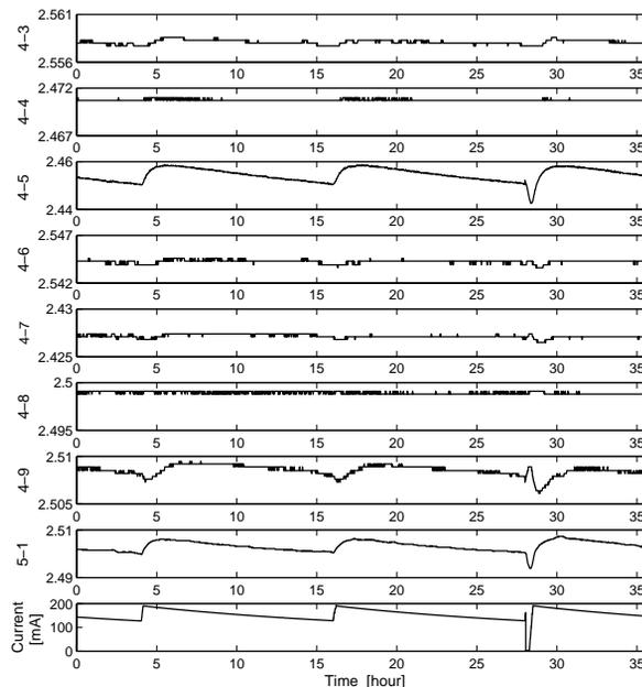
Figure 5: The measured vertical motion of vacuum chamber near BPM as the stored beam current changes for 36 hours. The vertical full scale in the graphs of BPM 4-5 and 5-1 is  $20 \mu\text{m}$ , others  $5 \mu\text{m}$ .
