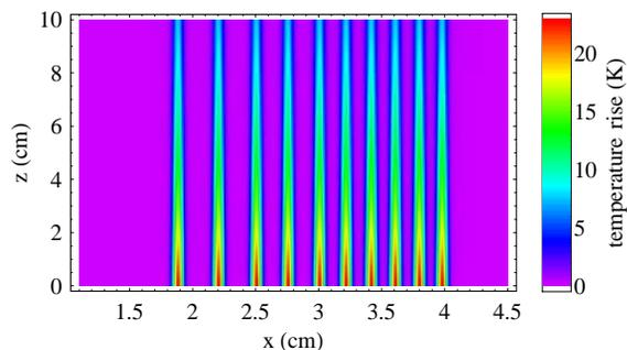
Figure 2:  $\Delta T$  in the first 10 cm in the carbon part of the TCDS during nominal ion operation.
