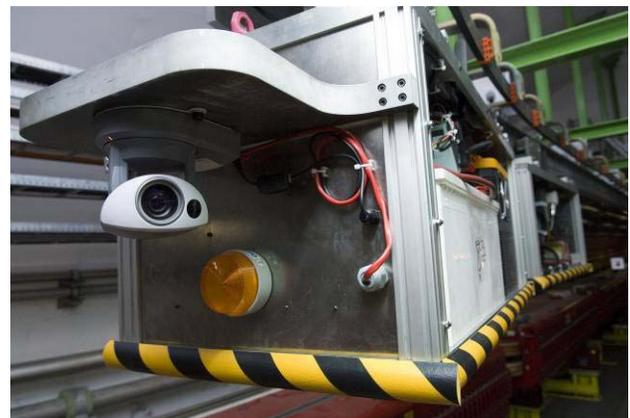
Figure 1: Remote inspection train on LHC monorail.
