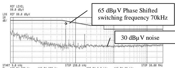
Fig. 9: Differential mode output voltage noise.
