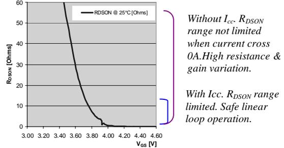
Fig. 5: MOSFET R<sub>DS(on)</sub> gain vs V<sub>GS</sub>.
