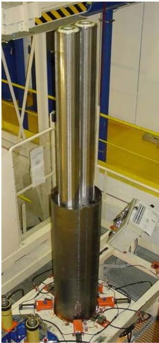
Figure 1: Yoke assembly around quadrupole apertures
