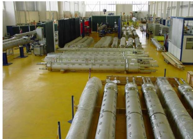
Figure 2: Quadrupole cold masses awaiting shipment at ACCEL
