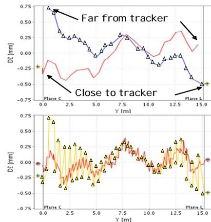
Figure 1: Top: the two vertical measurements, curve with markers from the non connection side. Bottom: the final result, points measured from both sides joined together, curve with markers represent the CERN measurements. The joined measurements in industry are also displayed, curve without markers. The crosses in circles at the ends of the measurements represent the position of the corrector magnets.
