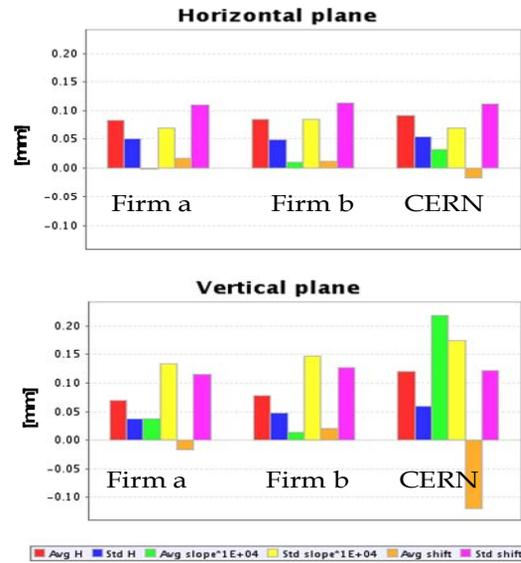
Figure 3: Saw tooth criteria, height (H) and slope applied to measurements in industry and at CERN. We see a significant change in the data for the CERN data, in the vertical plane only.
