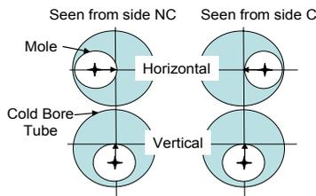
Figure 2: Mole centring errors in the two measurement planes: errors in the vertical plane not detectable.
