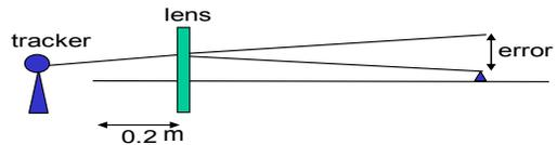
Figure 4: A convection zone at 0.2 m from the cold bore tube end acts as a lens and bends the laser beam used in the measurement. The convection zone is acting as a lens.
