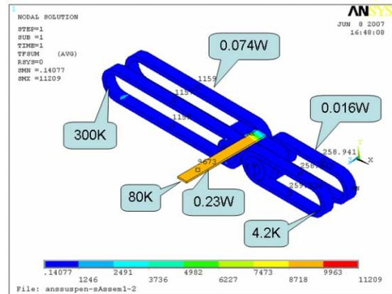
Figure 5: Heat flux of the suspension.
