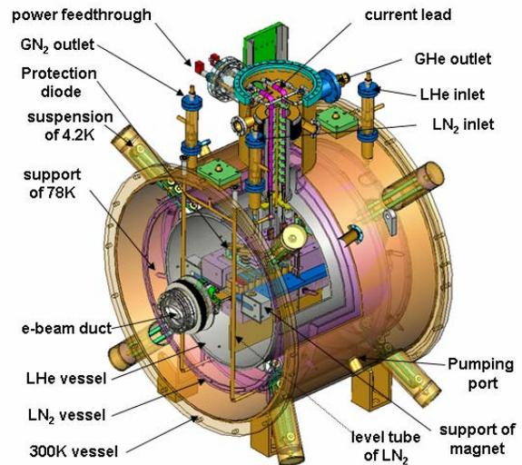
Figure 1: Structure of Superconducting magnet.
