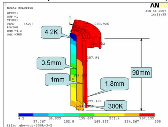
Figure 6: Temperature distribution and presents the structure of the transfer port.
