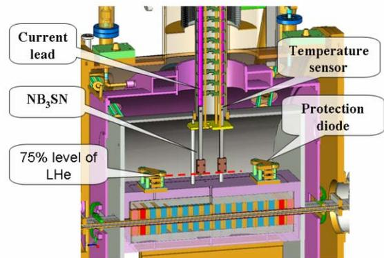
Figure 9: Nb<sub>3</sub>Sn bar was welded to immerse in the LHe to the 75% level in the helium vessel.
