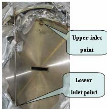
Figure 7: Designs of the LHe inlet tube.
