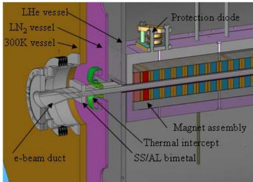
Figure 4: E-beam duct in the cryostat.
