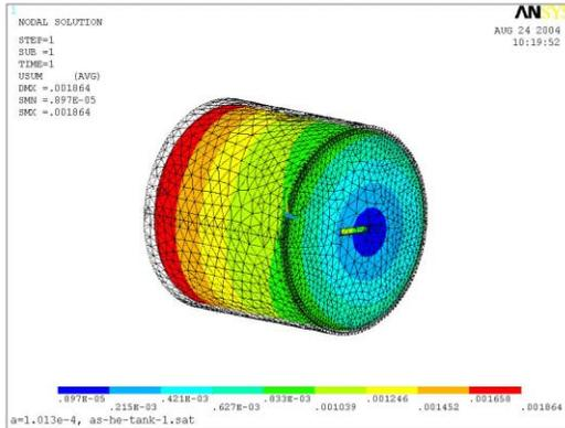
Figure 2: Reducing the diameter by 1.8 mm, when the helium vessel cooled to 4.2 K.
