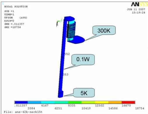
Figure 3: Heat flux of the service tower.
