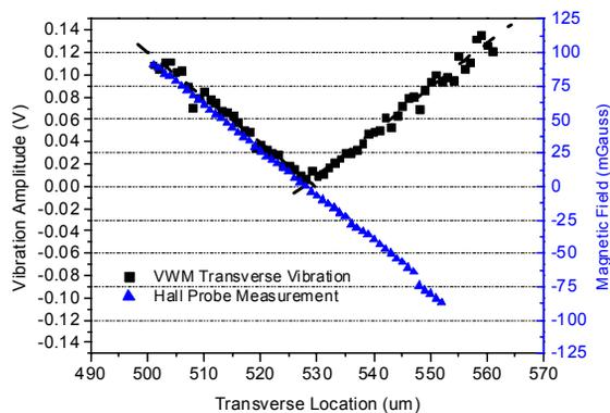
Figure 5: Comparison between VWM and Hall probe measurement for a Quadrupole Magnet.
