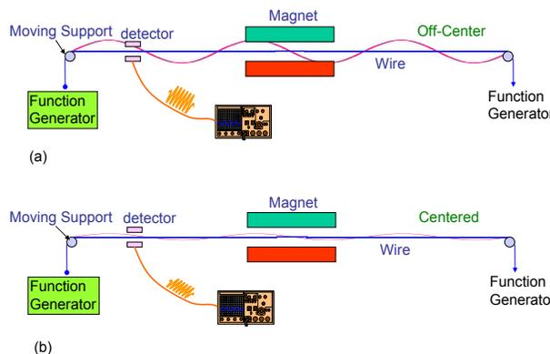
Figure 1: Vibrating Wire Method (courtesy of T. C. Fan).
