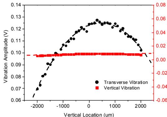
Figure 6: Vibration Amplitude vs. Vertical Location in measuring a Sextupole Magnet.
