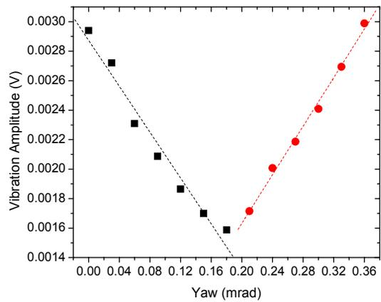
Figure 4: Vibration amplitude vs. yaw angles.
