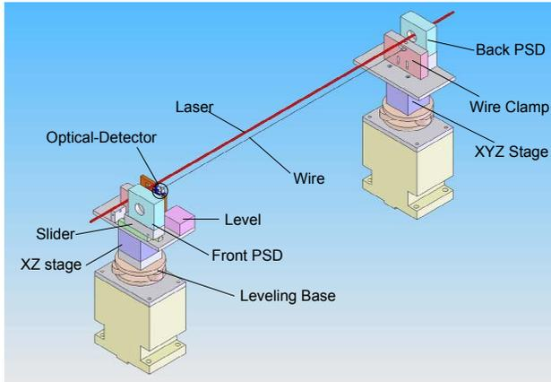
Figure 2: VWM and PSD system setup.
