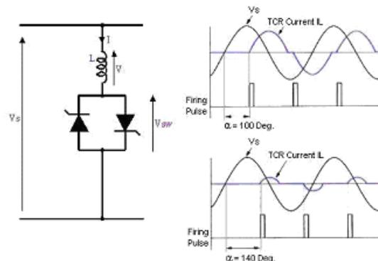
Fig. 1. TCR Configuration and Operation
