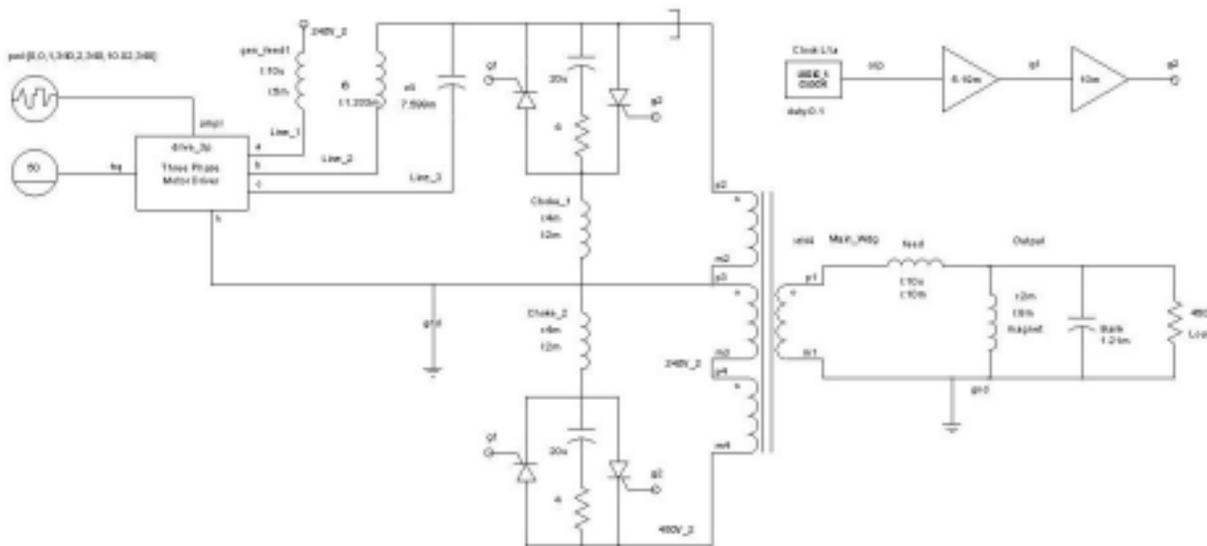
Fig. 2. Saber Schematic for the ISIS White Circuit with Static VAR Power Factor Correction
