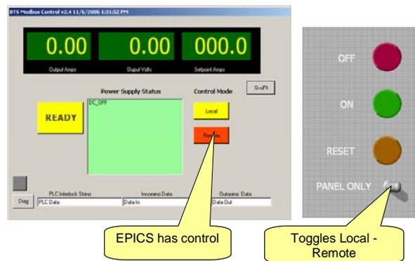
Figure 2: Display layout and relationship to physical buttons.
