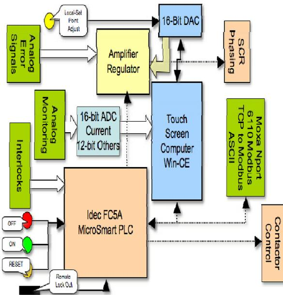
Figure 3: Interaction between control elements in the controller.
