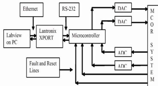
Figure 3: MCOR Digital Interface Block Diagram
