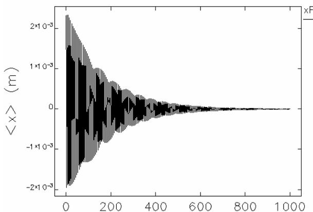
Figure 4: Beam trajectory tracking result with feedback on for a configuration with S3 pickup at S3 and kicker at S2.
