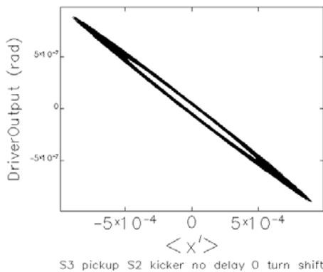
Figure 3: Kicker drive signal versus beam angle at the kicker with pickup at S3 and kicker at S2 with low kicker gain.
