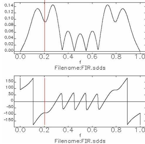
Figure 2: Amplitude (top) and phase (bottom) response of a 9-tap FIR filter generated with the TDLF method. The red vertical line indicates machine tune.
