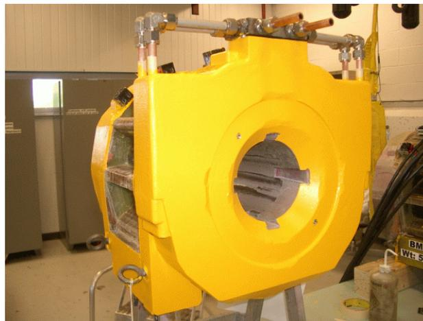
Figure 2 Corrector without BPM after potting and painting.
