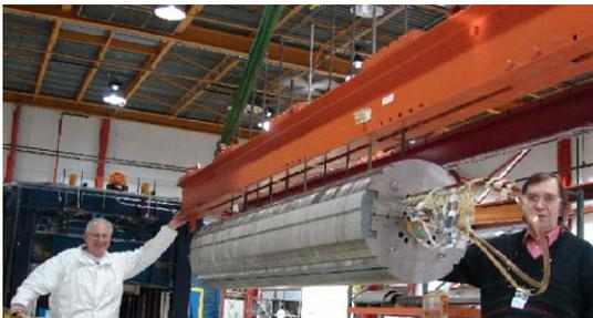
Figure 7: 2-m long mirror LM02 with PIT coil.
