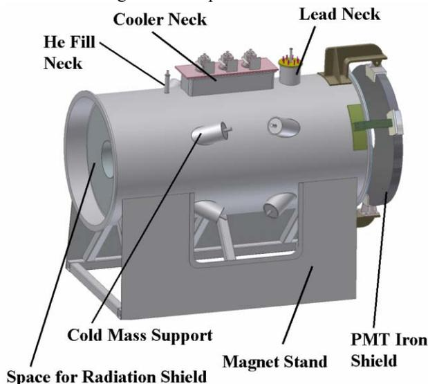
Figure 1: Spectrometer solenoid module 3D CAD image.
