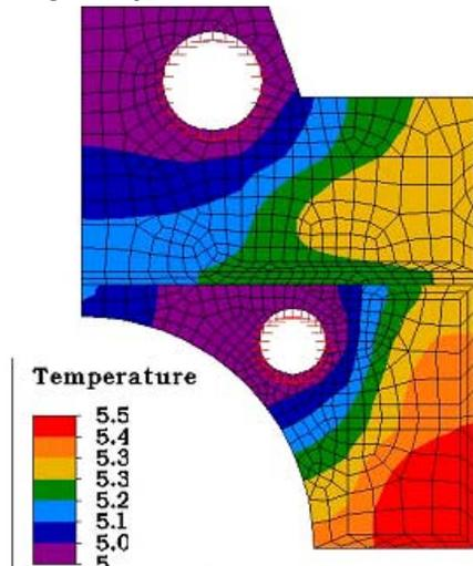
Figure 6: Temperature profile with supercritical cooling; the coil is dissipating 48 W/m at 9 T/s ramp rate.
