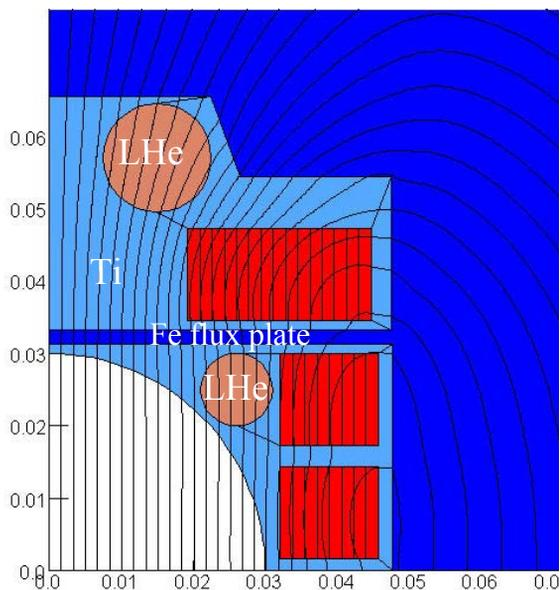
Figure 3: Structural design of rapid-cycling dipole.
