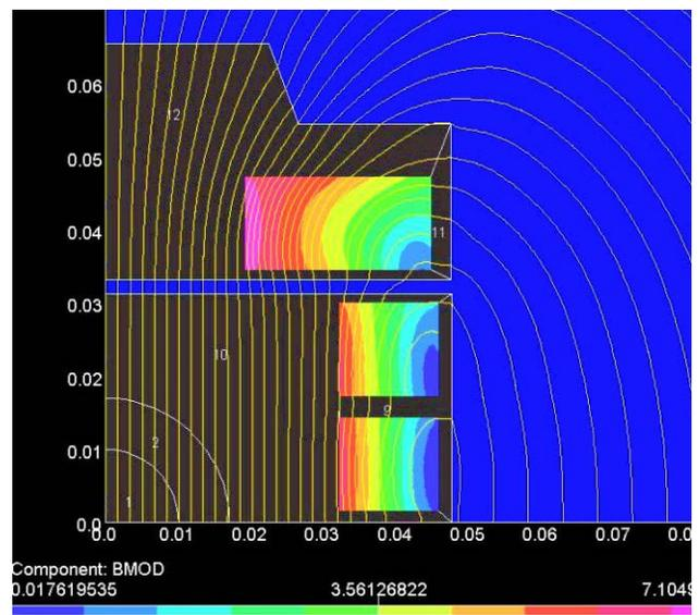
Figure 2: Field distribution in rapid-cycling block-coil dipole.  $B_{\text{mod}}$  is shown in coil blocks.
