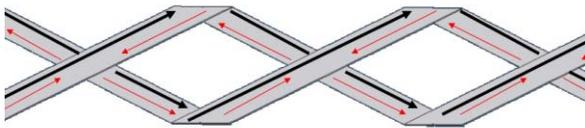
Figure 1: Induced coupling currents between adjacent strands when cable is face-on to flux (e.g.  $\cos \theta$ ).
