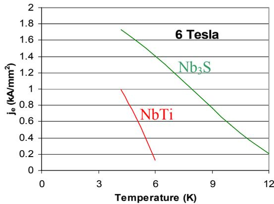
Figure 5:  $j_E$  vs.  $T$  for NbTi and  $Nb_3Sn$ .
