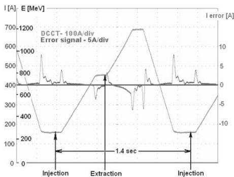
Figure 1: The ramping cycle, shown for the main power supply in terms of booster energy and magnet current, with injection at 273 MeV and extraction at 800 MeV.
