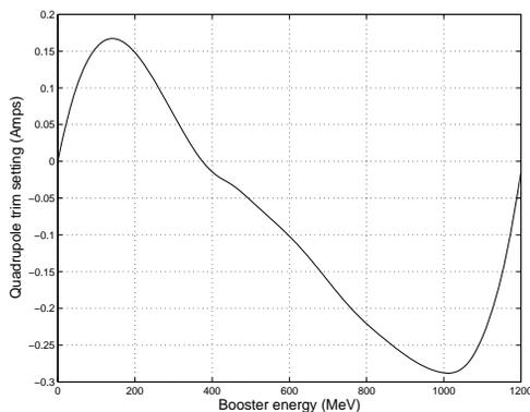
Figure 2: A defocusing quadrupole trim power supply current setting for the energy ramp cycle.
