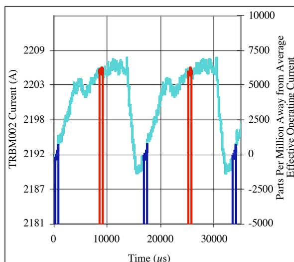
Figure 1: TRBM02 Current Ripple at 60 & 120Hz rep rate.
