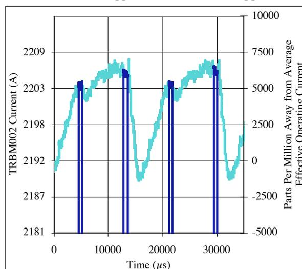
Figure 2: TRBM02 Current Ripple at 120Hz rep rate with delayed start of beam pulse.
