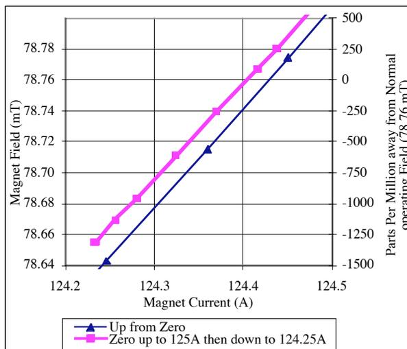
Figure 4: TDBM02 Hysteresis Error after a 0.5% variation up from and returning to normal current.
