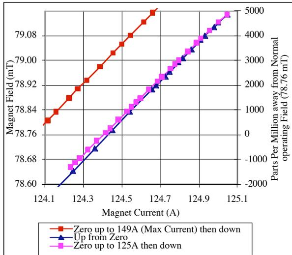
Figure 3: TDBM02 maximum hysteresis error at normal current.
