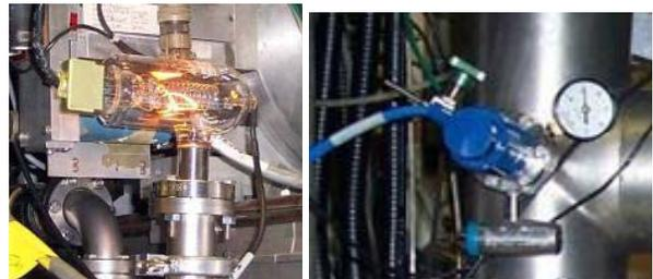
Figure 2: TA Bayard Albert Ion Gauge (left) and TB Granville Phillips Stabil-Ion Gauge (right).
