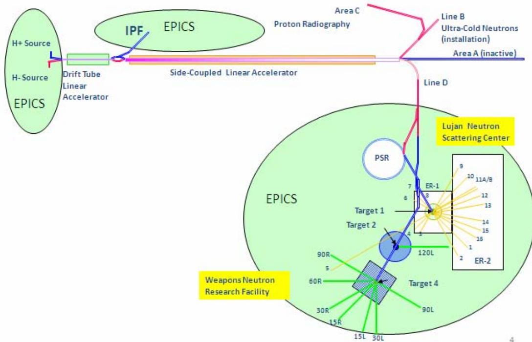
Figure 1: Schematic representation of LANSCCE accelerator and experimental areas.
