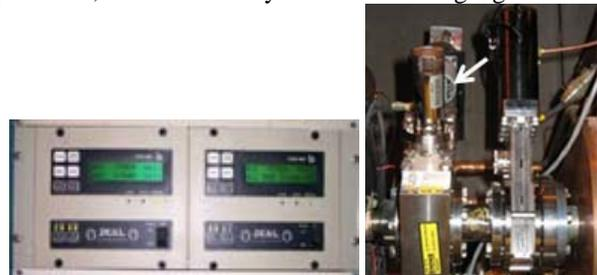
Figure 6: Varian Dual Ion Pump Controller (left) and a Stabil-Ion gauge intalled between SCL modules.
