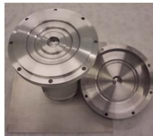
Figure 5: The cold model of the X-band switch cavity used for loss tangent measurements. The ferroelectric ring was placed into a circular sitting place shown in the photo.
