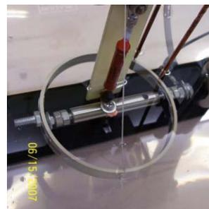
Figure 6: Experimental setup for the ring tunability measurements at high voltage. One can see the ring, RF probes and fixtures.
