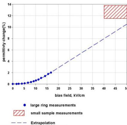
Figure 8: Perpendicular tunability for BSM-3 material prototype.
