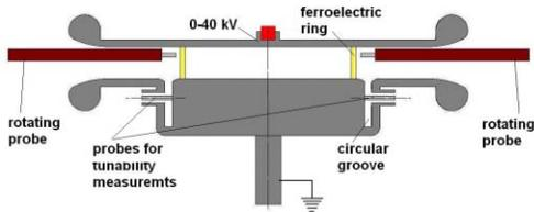
Figure 2: Schematic of the test cavity for the large ferroelectric ring measurements.
