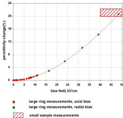
Figure 7: Parallel tunability for BSM-3 material prototype.
