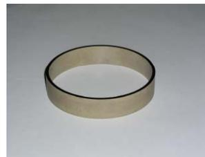
Figure 1: The large ferroelectric ring having the inner diameter of 104.2 mm, thickness of 2.6 mm, and length of 20.4 mm
