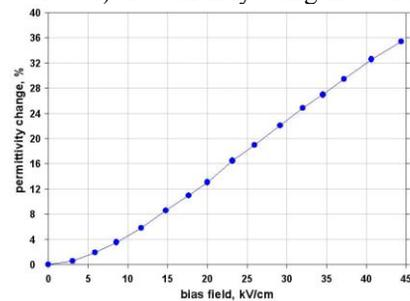
Figure 10: Parallel tunability for BSM-4 ferroelectric material. The ring inner diameter is 29 mm, thickness is 2 mm, and length is 7 mm.
