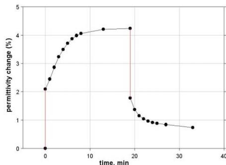
Figure 9: Long-term drift of the dielectric constant and hysteresis for BSM-3.
