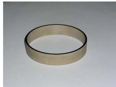
Figure 2: A sample of a metallized ferroelectric ring with a diameter of 104.2 mm, a thickness of 2.6 mm, and a length of 20.4 mm.
