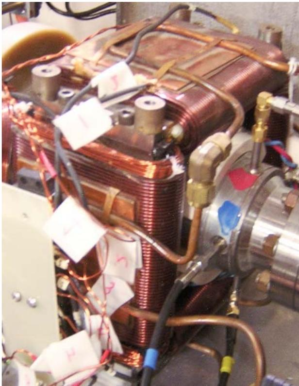
Figure 5: Combined Quadrupole/ Dipole in Injector.
