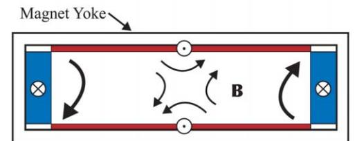
Rectangular Panofsky Quadrupole with Coil Currents (Looking Downstream, Focusing Electrons)
