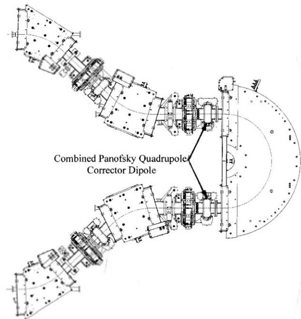
Figure 1: Arc 2, Showing Combined Magnets.
