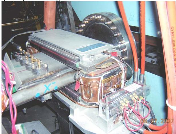
Figure 4: Combined Magnet in Arc Showing Corner Coils.
