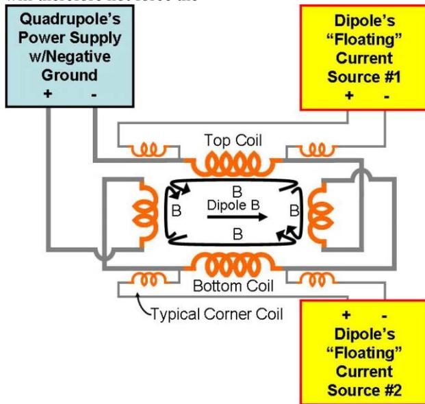
Figure 3: Quadrupole/Dipole Powering Schematic.
