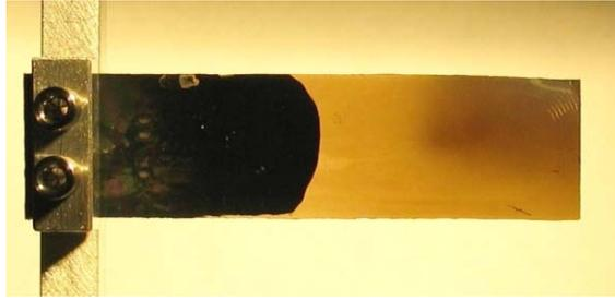
Figure 3: SNS 12x20 mm<sup>2</sup> foil after use. The image has been rotated 90° CCW from the true orientation. Damage is apparent in the figure upper right corner.
