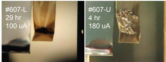
Figure 1: Nanocrystalline diamond foils irradiated at 100  $\mu\text{A}$  (left) and 180  $\mu\text{A}$  dc  $\text{H}^+$  at KEK. The foil is positioned to the right of a metal shield.
