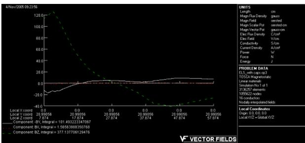
Fig. 5: Field along circulating beam axis upstream.
