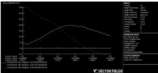
Fig. 6: Field along circulating beam axis downstream.
