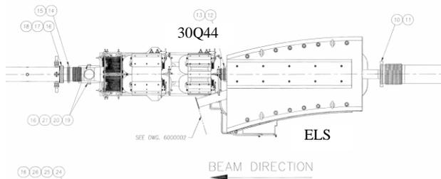
Fig. 1: Extraction septum and quad assembly (Courtesy of BNL/SNS design drawing and specifications)
