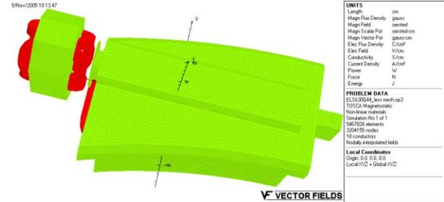
Fig. 7: 3D model for quad and ELS assembly.
