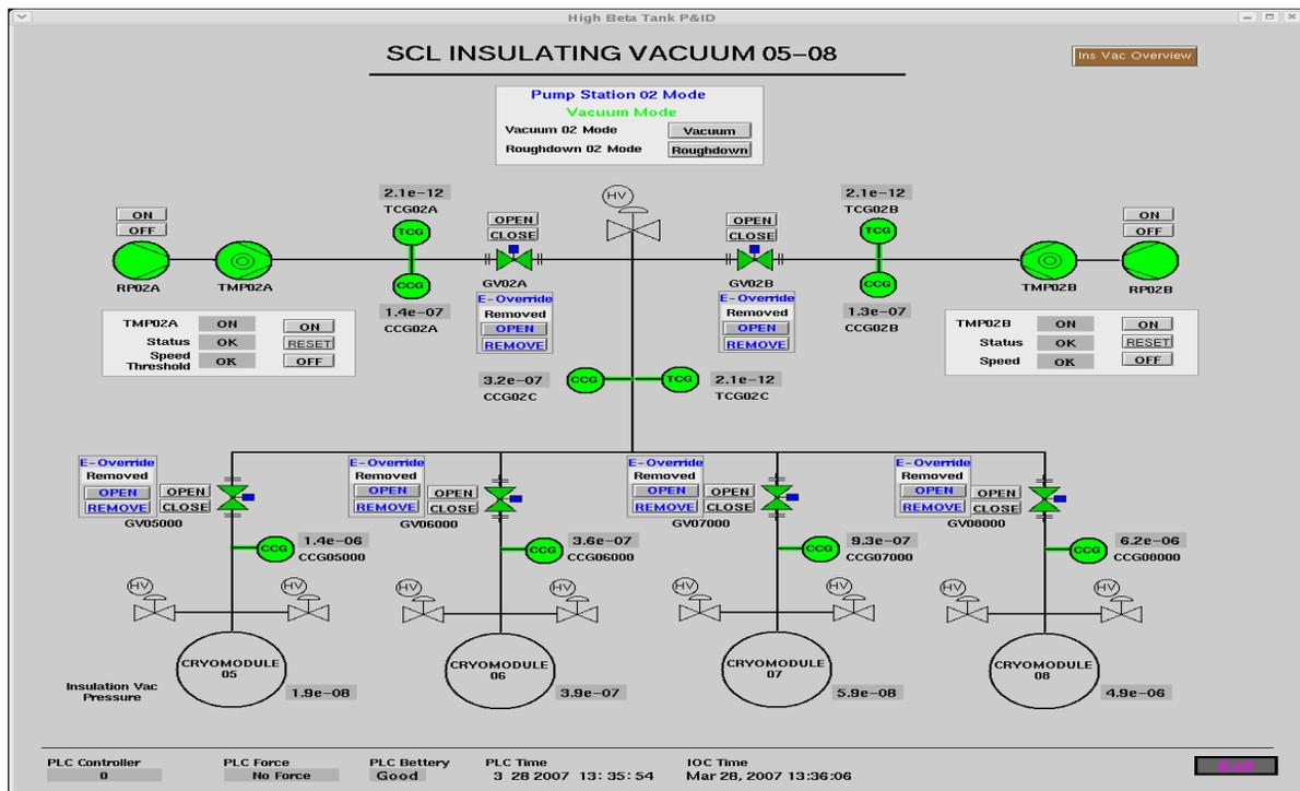
Figure 2 - IVS Control Screen for Cryomodules 5-8
