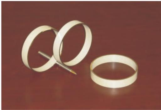
Figure 5. Large-diameter ceramic ring samples made of BST(M)3 ferroelectric. The ring diameter is 104.2 mm and the ring thickness is 2.6 mm.
