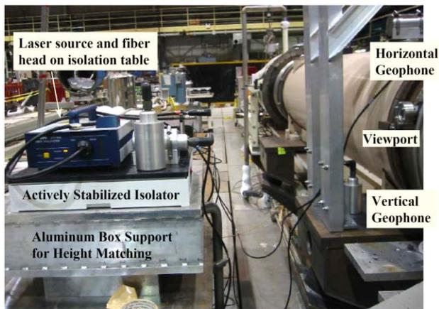
Figure 2: New laser setup for the CQS cold test.
