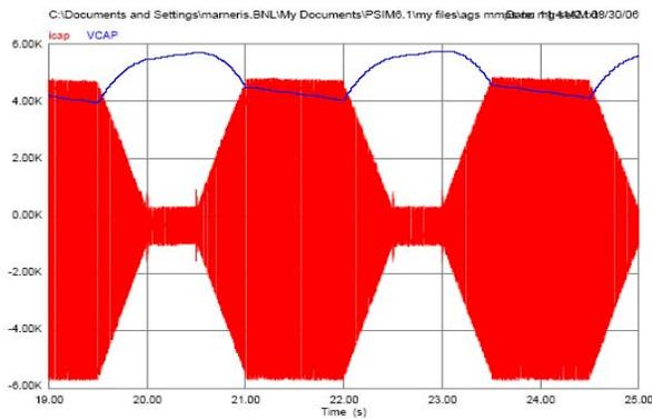
Figure 7: Capacitor voltage and current waveforms
