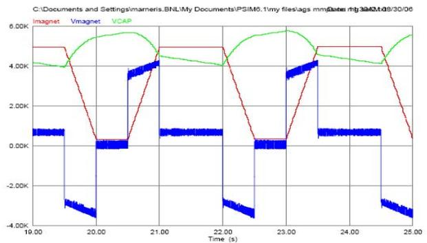
Figure 5: Magnet current, voltage and capacitor voltage
