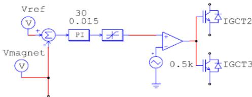
Figure 4: Two quadrant converter control system
