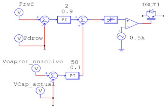
Figure 3: Buck converter control system
