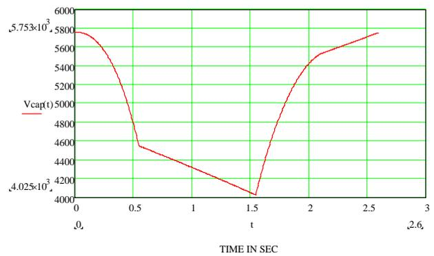
Figure 11: Calculated capacitor voltage waveform
