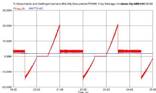
Figure 10: Average and pulsed power waveforms
