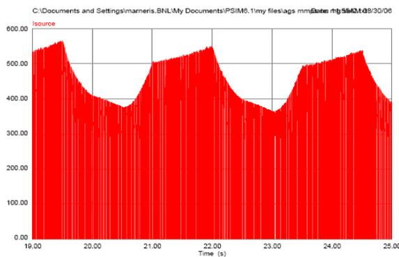
Figure 9: Rectifier dc current waveform
