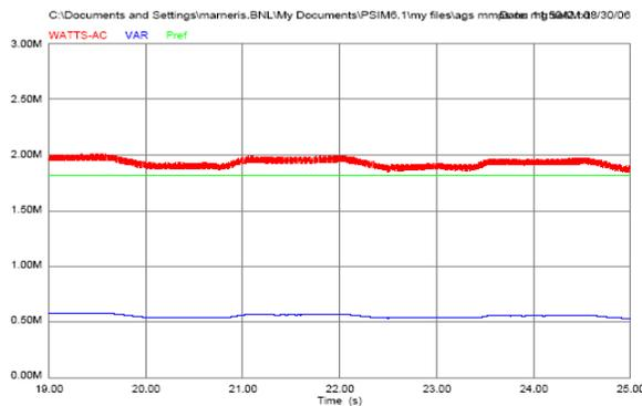
Figure 8: Real power, reactive and power reference
