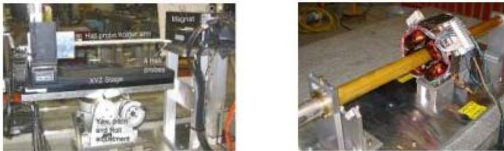
Figure 4. Magnetic measurements with rotating coil and Hall Probe array at Superconducting Magnet Division, BNL.
