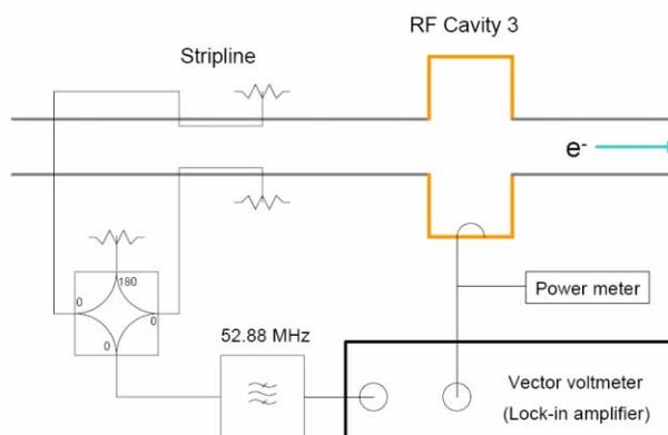
Figure 2. Experimental set-up for phasing of RF cavities of the X-ray storage ring. The change in the synchronous phase is monitored by a vector voltmeter.
