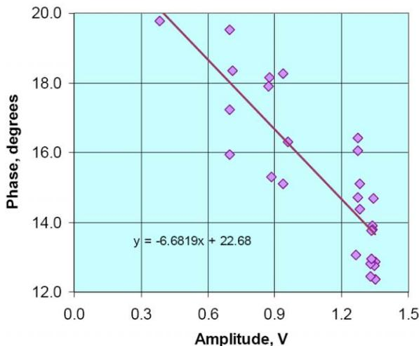
Figure 3. Dependence of phase difference between fields in the cavities 3 and 4 vs. amplitude of cavity 4 voltage.
