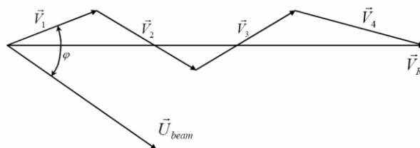
Figure 1. Vector diagram of the accelerating voltages and electron beam current.
