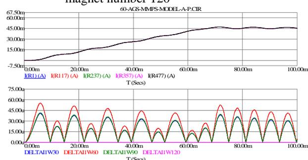
Figure 8: Magnet current waveforms and magnet current differences
