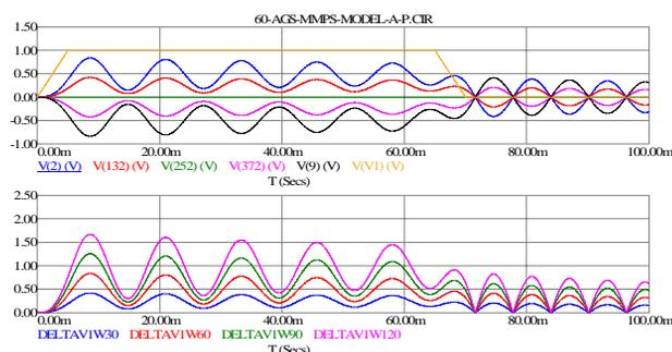
Figure 9: Magnet current waveforms and magnet current differences
