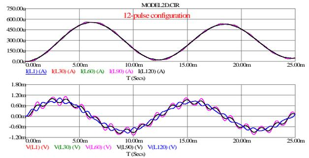
Figure 4: Magnet current and voltage waveforms of first 25 ms with 720 Hz input under 12-pulse configuration
