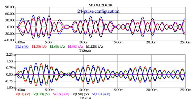
Figure 6: Magnet current and voltage waveforms of first 25 ms with 720 Hz input under 24-pulse configuration
