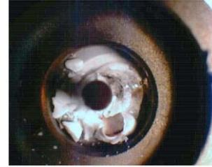
Figure 5: LER BPM feedthrough after overheating.
