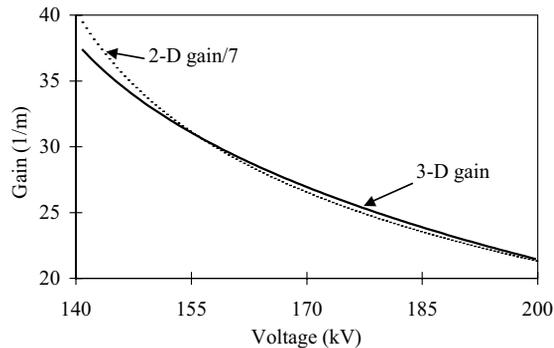
Figure 5: 3-D field gain coefficient for the amplifier mode is a factor of seven smaller than 2-D gain coefficient.
