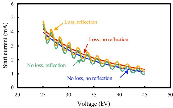
Figure 4: Start current with and without losses and reflections as a function of voltage for the parameters shown in Table 1. In this regime the losses and reflections do not have a strong impact on device operation, however, at shorter wavelengths it is expected that losses will raise the start current substantially.
