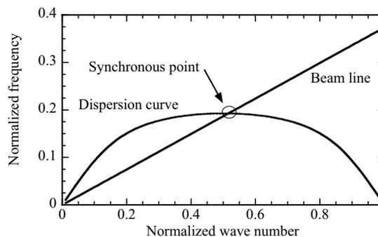
Figure 2: Dispersion relation for the grating used in the Dartmouth College experiments, grating parameters listed in Table 1. The intersection of the dispersion curve and beam line determines the operating frequency and wavenumber at which the phase velocity of the evanescent wave matches the velocity of the electron beam. The slope of the dispersion curve at the intersection determines the group velocity of the evanescent wave,  $v_g = \frac{\partial \omega}{\partial k}$ .
