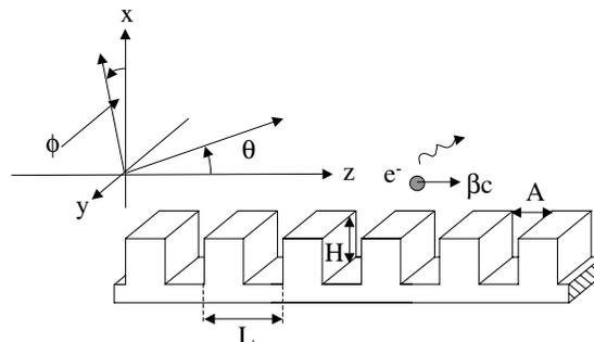
Figure 1: The lamellar grating geometry used in the two and three dimensional theories shown with an electron ( $e^-$ ) and emitted photon (squiggly line).
