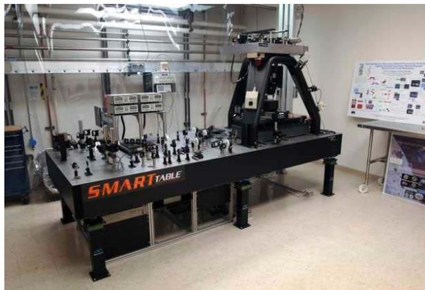
Figure 4. The JLab Laser Microengineering Station. This system provides state of the art positioning of an intensity controlled laser beam as well as write velocity control to ensure equal exposure. The system is programmable from converted CAD drawing files. Although we do not yet have the UV FEL operational we have demonstrated high power upconversion to the UV of 1 micron lasing which can be used as a source at the required powers.
