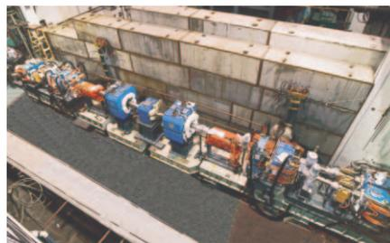
Figure 2: The IR with conventional magnets: the dipole in the middle is used in the BSR to connect outer half rings. Two quadrupoles on each side of the dipole are used in the collision mode for squeezing the beta function at IP.
