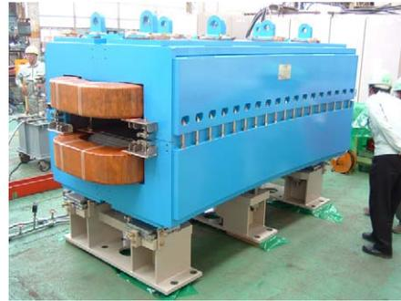
Figure 4: Bending magnet for the 3-GeV synchrotron.
