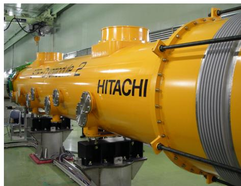
Figure 7: STF cryomodule as completed.
