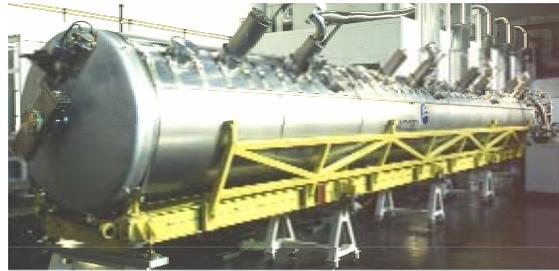
Figure 1: LEP module housing 4 4cell cavities.
