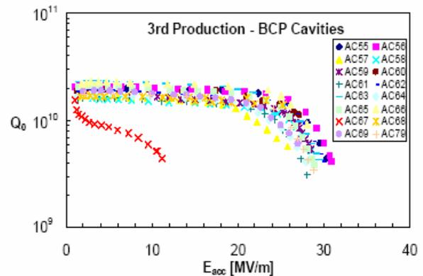
These results show that a mean value of 23 MV/m with a quality factor of above  $1.0 \cdot 10^{10}$  can be achieved with industrially consolidated cavity manufacturing procedures and the surface preparation sequence developed at DESY. Based on these results European industry is ready to provide cavities as well as complete modules following the DESY established procedures with guaranteed parameters.
