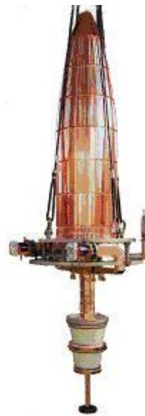
Figure 6: 5-GHz, 500-kW klystron E3762.
