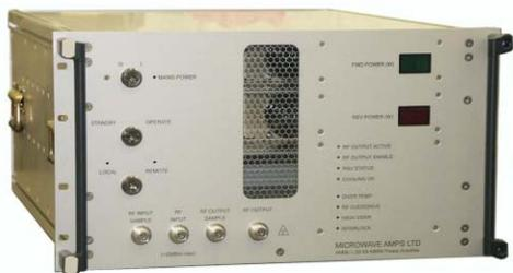
Figure 4: 650 watt driver developed for XFEL by Microwave Amplifiers Ltd [5].
