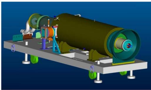
Figure 3: Schematic view of Thales TH1802 in horizontal format to facilitate placing in a tunnel [4].
