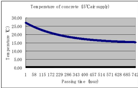
Figure 4: Temperature of tunnel concrete during maintenance of accelerator.
