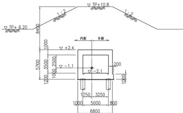
Figure 1: Cross-section of J-PARC 50GeV synchrotron tunnel
