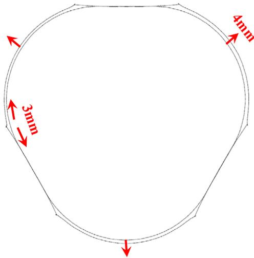
Figure 5: Transformation of the ring tunnel.
