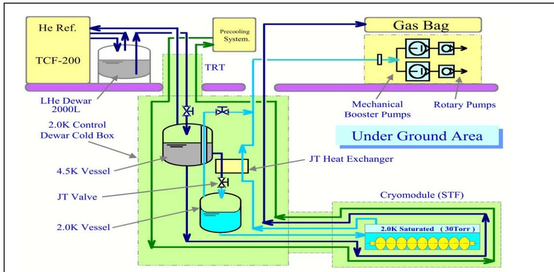
Figure 1: Schematic Flow Diagram of STF Cryogenic System
