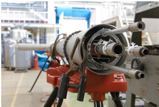
Figure 3: High Performance Transfer Line Designed by KEK.
